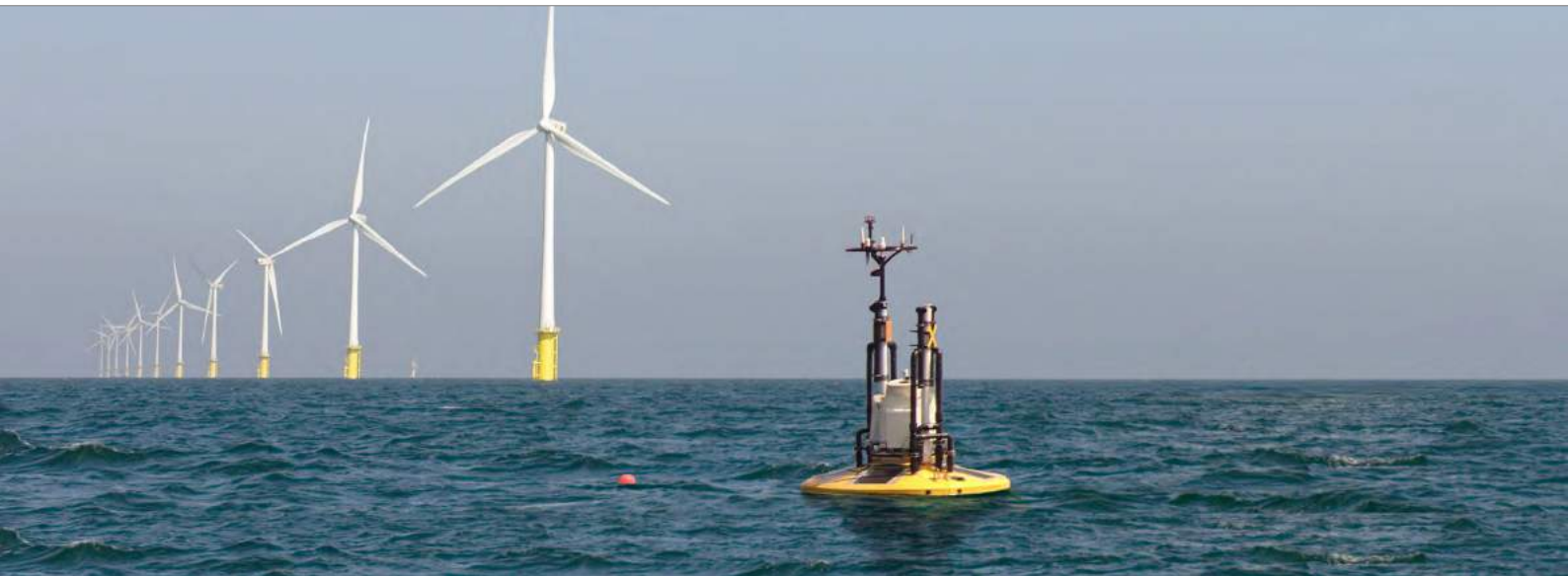
Fugro's Seawatch Lidar buoy for measuring wind profiles and waves.
